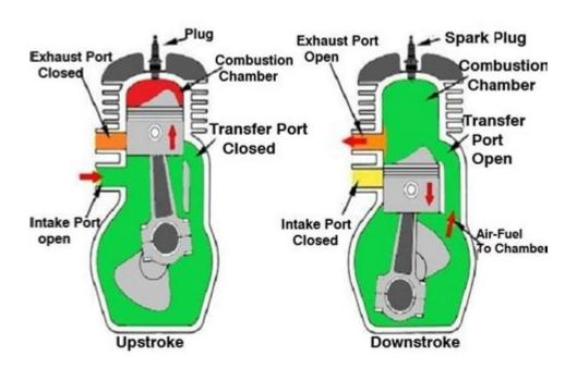
How does a 2 stroke engine work is a question many people ask when trying to understand the mechanics behind this type of internal combustion engine. Unlike its four-stroke counterpart, the two-stroke engine completes a power cycle with just two strokes of the piston, allowing for a simpler and lighter construction. This article will delve into the inner workings of a two-stroke engine, its components, advantages, disadvantages, and applications.
