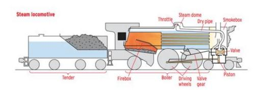
**How do steam locomotives work**? Steam locomotives are fascinating machines that played a vital role in the development of transportation during the 19th and early 20th centuries. Their engineering marvel combines physics, chemistry, and mechanical innovation to create powerful vehicles capable of hauling heavy loads across vast distances. In this article, we will delve into the intricate workings of steam locomotives, exploring their components, operation, and the science behind steam power.
