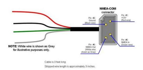
**GPS** tracker wiring diagram is an essential component for anyone looking to install a GPS tracker in their vehicle, boat, or any other asset that requires tracking. Understanding the wiring diagram helps users connect the device correctly and ensures optimal performance. In this article, we'll explore the components of a GPS tracker wiring diagram, how to read it, the installation process, and some common troubleshooting tips to keep your GPS tracking system running smoothly.
