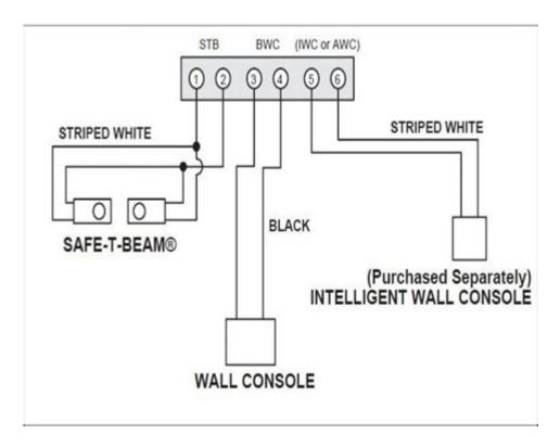
Garage door safety sensor wiring diagram plays a crucial role in ensuring the safe operation of automatic garage doors. These sensors are designed to detect objects in the path of the closing garage door, preventing accidents and injuries. Understanding how to wire these sensors correctly is essential for both safety and functionality. This article will explore the components of garage door safety sensors, the wiring process, troubleshooting common issues, and tips for ensuring proper operation.
