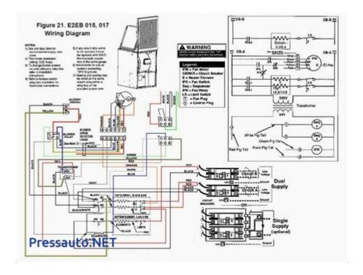
**Gas furnace wiring diagram** is an essential tool for understanding the electrical system of your gas furnace. Whether you are a homeowner looking to troubleshoot issues or a technician performing maintenance, having a clear wiring diagram can make all the difference. This article will delve into the components of a gas furnace, the importance of a wiring diagram, how to read one, and tips for safe handling and troubleshooting.
