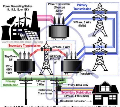
Typical AC Power Supply System (Generation, Transmission and Distribution)
