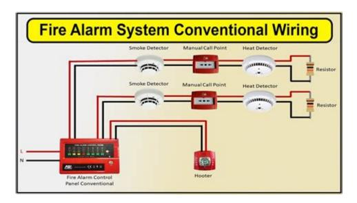
Fire alarm cable installation guide is essential for ensuring the safety and reliability of fire detection systems in both residential and commercial properties. Proper installation techniques not only enhance the performance of fire alarm systems but also comply with building codes and safety regulations. This comprehensive guide will walk you through the crucial steps, considerations, and best practices for installing fire alarm cables effectively.
