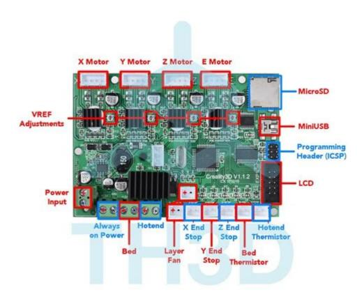
Ender 3 wiring diagram is an essential aspect of understanding and maintaining your Creality Ender 3 3D printer. As a popular choice among hobbyists and professionals alike, the Ender 3 features a relatively simple wiring setup that is crucial for its operation. In this article, we will explore the components involved, how to read and interpret the wiring diagram, common issues related to wiring, and tips for troubleshooting and modifications.
