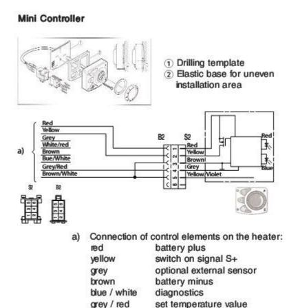
Espar D2 wiring diagram is an essential aspect of understanding how to install and troubleshoot the Espar D2 air heater, a popular choice for heating vehicles and small spaces. The D2 heater is known for its efficiency and reliability, making it a go-to option for campers, truckers, and outdoor enthusiasts. This article will delve into the various components of the Espar D2 heater, the significance of the wiring diagram, and a comprehensive guide on how to wire it effectively.
