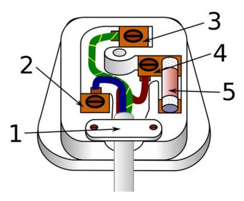
**Electrical plug wiring diagram** is an essential concept for anyone working with electrical devices or installations. Understanding how to read and create wiring diagrams can significantly enhance safety and efficiency when working with electrical systems. This article will explore the components of electrical plugs, various types of plugs, the importance of wiring diagrams, and a step-by-step guide on how to wire a plug correctly.
