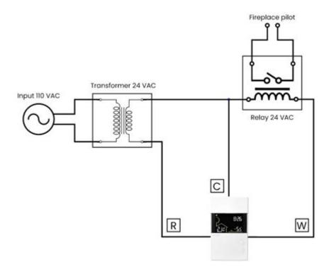
**Electric fireplace heater wiring diagram** serves as a crucial guide for both professionals and DIY enthusiasts who wish to install or troubleshoot electric fireplace heaters. Understanding the wiring diagram not only ensures safe installation but also helps in the efficient operation of the heater. This article will delve into the components of an electric fireplace heater, the importance of wiring diagrams, and a step-by-step guide for wiring an electric fireplace heater.
