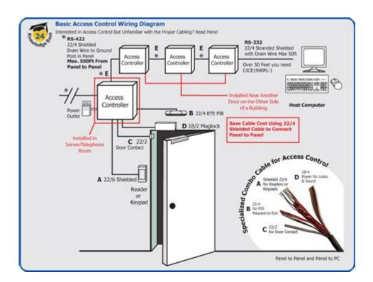
**Door access control system wiring diagram** is an essential aspect of modern security solutions, enabling businesses, institutions, and residential properties to efficiently manage who can enter specific areas. A proper understanding of the wiring diagram is crucial for both installation and troubleshooting of access control systems. This article will provide a comprehensive overview of the components, wiring methods, and considerations involved in setting up a door access control system.
