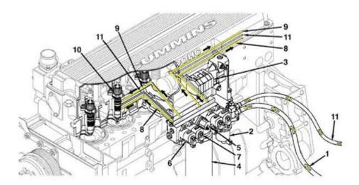
**Cummins M11 fuel system diagram** is an essential aspect for understanding how this robust engine operates. The Cummins M11 engine is widely used in various applications such as trucks, buses, and heavy machinery, making it important for technicians and operators to have a clear understanding of its fuel system. This article will delve into the intricacies of the Cummins M11 fuel system, illustrating its components and how they interact with each other to deliver optimal performance.
