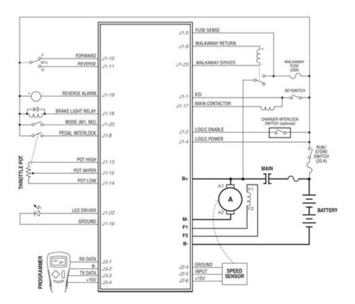
CURTIS 1268 CONTROLLER WIRING DIAGRAM IS AN ESSENTIAL RESOURCE FOR ANYONE WORKING ON ELECTRIC VEHICLES OR MATERIAL HANDLING EQUIPMENT THAT EMPLOYS THE CURTIS 1268 MOTOR CONTROLLER. UNDERSTANDING HOW TO PROPERLY CONNECT AND WIRE THIS CONTROLLER CAN HELP ENSURE THE SAFE AND EFFICIENT OPERATION OF ELECTRIC POWERTRAINS. IN THIS ARTICLE, WE WILL DELVE INTO THE SPECIFICS OF THE CURTIS 1268 CONTROLLER WIRING DIAGRAM, ITS COMPONENTS, AND BEST PRACTICES FOR INSTALLATION AND TROUBLESHOOTING.
