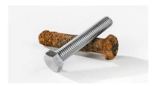
**Corrosion resistance of metals and alloys** is a critical aspect of material selection in various industries, including construction, automotive, aerospace, and marine applications. Corrosion can lead to significant economic losses, safety hazards, and environmental concerns. Understanding the mechanisms of corrosion and how different metals and alloys can resist it is essential for engineers and manufacturers to make informed decisions.
