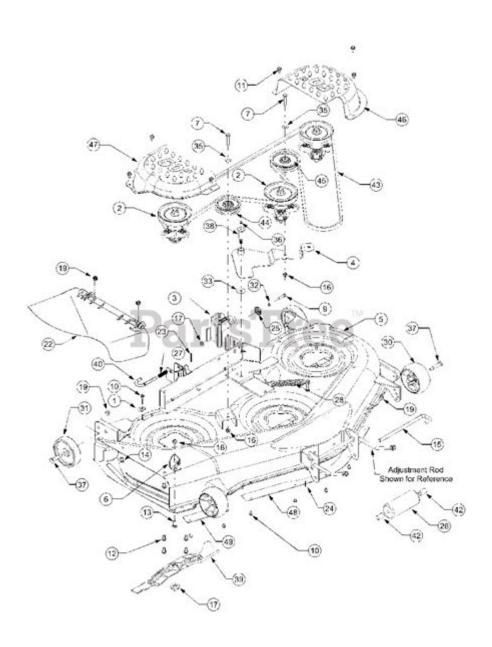
**Cub Cadet 50 inch mower deck parts diagram** is an essential resource for anyone who owns or maintains a Cub Cadet lawn mower equipped with a 50-inch cutting deck. Understanding the parts of your mower deck is crucial for proper maintenance, repairs, and ensuring that your mower functions efficiently. In this article, we'll delve into the components of the Cub Cadet 50-inch mower deck, explore how to read the parts diagram, and provide tips for maintenance and repair.
