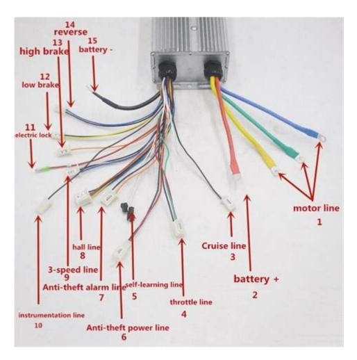
Controller wiring e-bike throttle wiring diagram is an essential aspect of building or upgrading an electric bike (e-bike). Understanding how to wire the throttle to the controller is crucial for ensuring proper functionality and safety. This article will guide you through the various components involved, the wiring process, and some troubleshooting tips to help you create an efficient e-bike system.
