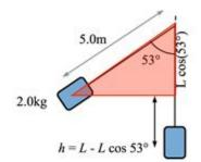
We can find the height of the pendulum bob relative to the bottom of its swing by using trigonometry. The length of the short side of the triangle (shown in red) is  $L\cos 53^\circ$ . The height b is the full length L less this leg of the triangle.
