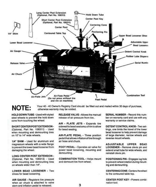
Coats 1010 tire machine manual is an essential resource for anyone involved in tire changing and repair. This manual provides comprehensive guidance on operating the Coats 1010 tire machine, ensuring that technicians can effectively and safely perform tire service tasks. In this article, we will delve into the key features of the Coats 1010 tire machine, discuss its operation, maintenance tips, troubleshooting techniques, and the importance of the manual for both new and experienced technicians.
