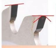
Triple-Chip Grind (TCG) teeth have beveled corners. On the blade, they alternate with FTG teeth. TCG teeth don't have scoring bevels, so they're very durable. They're used on glue-line rip blades and blades for melamine board, laminates and other manufactured materials when tooth durability is most important.
