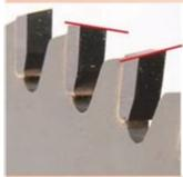
Alternate Top Bevel (ATB) teeth cut like knives, scoring the wood to minimize tear-out. Bevel angles vary: Increasing the angle improves cut quality but reduces durability. ATB teeth are used on crosscut, general-purpose and some rip blades.
