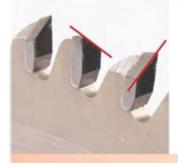
High-Angle Alternate Top Bevel (Hi-ATB) teeth have steep bevel angles (30 to 40 degrees) to cut melamine perfectly without tearing out the paper-thin face veneers. This tooth configuration is also great for hardwood plywood. These steeply beveled teeth are less durable than regular ATB teeth, though.
