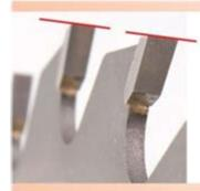
Flat Top Grind (FTG) teeth plow through the wood. They're primarily used on rip blades, where a fast feed rate is important to prevent overheating and bottom-side tear-out isn't an issue because the cut runs parallel to the wood fibers.
