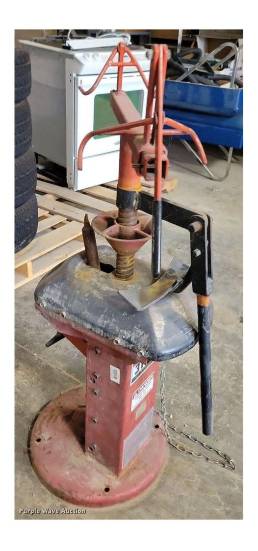
Coats 310 Manual Tire Changer is a widely recognized piece of equipment in the automotive industry, particularly for tire shops and garages. This manual tire changer stands out for its simplicity, durability, and efficiency, making it a go-to option for professionals and enthusiasts alike. In this article, we will explore the features, benefits, and operational guidelines of the Coats 310, as well as some tips for maintenance and troubleshooting.
