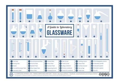
**Chemistry lab glassware names** are essential to the success of any scientific experiment. Whether you're a student, a researcher, or a professional chemist, understanding the various types of glassware used in chemistry labs can significantly enhance your efficiency and accuracy. This article will delve into the different types of glassware commonly found in chemistry labs, their specific uses, and important considerations when selecting and using them.
