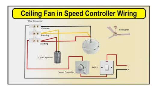
Ceiling fan speed control switch wiring diagram is an essential topic for anyone looking to install or upgrade their ceiling fan system. Understanding how to wire a ceiling fan speed control switch correctly can significantly enhance the functionality of your ceiling fan, allowing you to adjust the speed according to your preference. This article will explore the necessary components, wiring configurations, and safety measures to consider when working with ceiling fan speed control switches.
