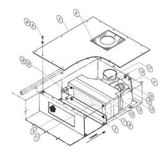
Figure 1. FWD Evaporator Assembly (STD)
