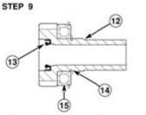
Remove and discard the oil seal (13) from the PTO drive shaft (12). Remove the snap ring (14) and use a hydraulic press to remove the bearing (15) from the PTO drive shaft (12).
