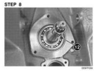
Remove the PTO drive shaft (12).
