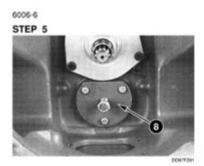
Use the removal plate (8), refer to Tools to be Made, Page 3, to remove the PTO driven shaft from the bearing.
