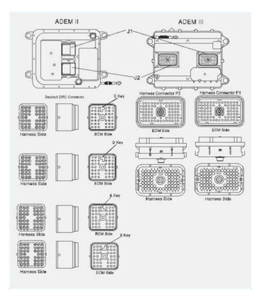
Cat 40 Pin ECM Wiring Diagram
