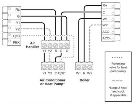
NOTE Do not connect any jumper wires between Rc and Rh. ecobee does this automatically. The R wire needs to go into the Rc terminal on your ecobee.
