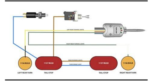
Brake light wiring diagram is an essential aspect of automotive repair and maintenance. Understanding how the brake light system operates and how to troubleshoot it can save you time, money, and ensure your vehicle remains safe on the road. This article will delve into the components of a brake light wiring system, the common wiring diagrams, troubleshooting tips, and more.
