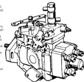
The purpose of the fuel injection pump is to deliver an exact metered amount of fuel, under high pressure, at the right time to the injector. The injector, unlike in a gasoline engine, injects the fuel directly into the cylinder or a prechamber connected to the cylinder.
