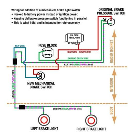
**Brake light switch wiring diagram** is an essential component for understanding how your vehicle's brake light system operates. The brake light switch is a crucial part of your vehicle's electrical system, as it controls the activation of your brake lights whenever the brake pedal is pressed. In this article, we will explore the wiring diagram for the brake light switch, its functions, the components involved, troubleshooting tips, and how to replace the switch if necessary.
