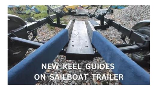
Boat trailer keel guides are essential components for boat owners who frequently transport their vessels on trailers. These guides assist in aligning the boat properly on the trailer and serve as a protective measure to prevent damage during loading and unloading. Understanding the purpose, types, installation, and maintenance of keel guides can greatly enhance the boating experience.
