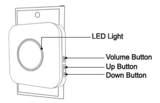
bitiwend door chime manual is an essential guide for anyone looking to set up or troubleshoot their Bitiwend door chime system. Whether you've recently purchased a Bitiwend door chime or are trying to fix an existing installation, understanding the manual can help you maximize the functionality of this convenient device. In this article, we will cover everything you need to know about the Bitiwend door chime, including setup instructions, troubleshooting tips, and maintenance advice.
