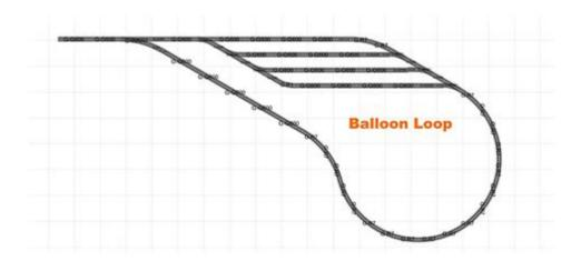
**Balloon loop railway track design guide** is an essential resource for engineers and railway planners looking to optimize their railway systems. Balloon loops are critical components in the design of railways, allowing for the efficient turnaround of trains, especially in areas where space is limited. This guide will explore the principles of balloon loop design, the advantages of using balloon loops, and practical considerations for implementation.
