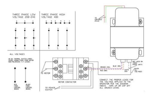
Baldor motors wiring diagram is an essential resource for anyone looking to install, troubleshoot, or maintain Baldor electric motors. Understanding the wiring configurations and electrical connections of these motors can significantly enhance operational efficiency and safety. In this article, we will explore the various aspects of Baldor motors wiring diagrams, including their components, types, and how to read and interpret them effectively.
