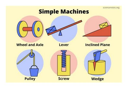
**Basic machines** are fundamental devices that help us perform work more efficiently by changing the direction or magnitude of a force. These machines are the building blocks of more complex machinery and play a crucial role in various applications, from simple household tasks to intricate industrial processes. Understanding how basic machines function can enhance our appreciation of technology and improve our ability to solve practical problems.
