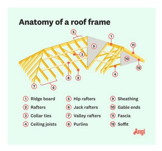
Anatomy of a roof frame is a critical aspect of any building's structure. Understanding the components and layout of a roof frame can help homeowners, builders, and architects make informed decisions about construction, maintenance, and repairs. This article will delve into the various elements that comprise a roof frame, their functions, and the overall significance of each component in ensuring the stability and durability of a building.
