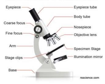
Anatomy of a Microscope: The microscope is an essential instrument in various scientific fields, providing the ability to observe and study objects at a magnified scale. Understanding the anatomy of a microscope is vital for both novice and experienced users, as it enhances their ability to utilize this tool effectively. This article will delve into the various components of a microscope, their functions, and how they work together to provide a clear and magnified view of microscopic specimens.
