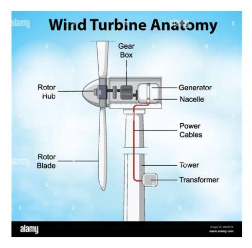
**Anatomy of a Wind Turbine**: Understanding the Key Components and Their Functions
