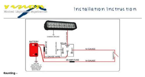
dount light bar in desired location, keep bottom base nuts snug but don't tighten. Adjust bar so it is centered on
