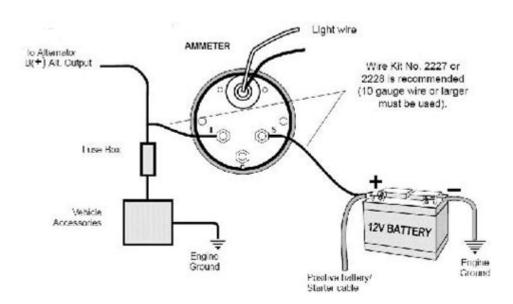
**Amp meter ammeter gauge wiring diagram** is an essential aspect for anyone looking to measure electrical current in automotive or industrial applications. Understanding how to wire an ammeter correctly is crucial for accurate readings and safe operation. In this article, we will delve into the significance of ammeters, explore the different types, provide a detailed wiring diagram, and offer tips for effective installation.
