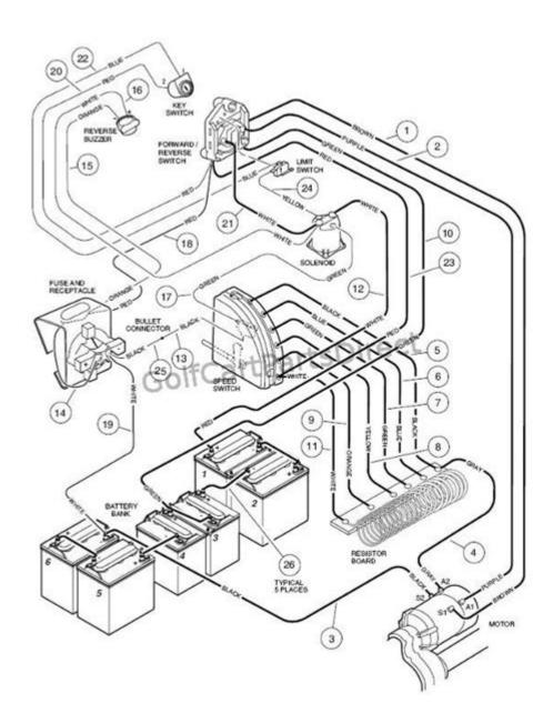
**36 volt golf cart motor wiring diagram** is essential for anyone looking to troubleshoot, repair, or upgrade their golf cart's electrical system. Understanding the wiring diagram helps ensure that all components work harmoniously and can prevent future issues. This article will delve deep into the intricacies of the 36 volt golf cart motor wiring diagram, covering its components, the wiring process, and common troubleshooting tips.
