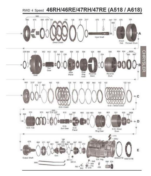
**46RE transmission parts diagram** is an essential tool for anyone involved in the maintenance, repair, or modification of Chrysler's 46RE automatic transmission. This transmission was prominently used in various Dodge and Chrysler models from the early 1990s to the early 2000s, particularly in trucks and vans. Understanding the components and their functions as depicted in the parts diagram can facilitate effective troubleshooting and repairs, ultimately extending the lifespan of the vehicle.
