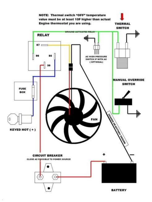
3 wire radiator fan wiring diagram is an essential topic for those involved in automotive repair and maintenance. Understanding how to wire a radiator fan correctly can prevent many issues, such as overheating and engine damage. A 3 wire radiator fan system typically consists of three wires: power, ground, and a signal wire. This article will explore the purpose of each wire, how to interpret the wiring diagram, and provide a step-by-step guide on how to wire a 3 wire radiator fan effectively.
