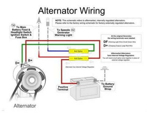
**3 Pin Alternator Wiring Diagram** is an essential topic for automotive enthusiasts and mechanics alike. Understanding how to wire a 3 pin alternator is crucial for ensuring proper functionality and longevity of the vehicle's electrical system. In this article, we will delve into the intricacies of a 3 pin alternator wiring diagram, discussing its components, wiring process, and tips for troubleshooting potential issues.
