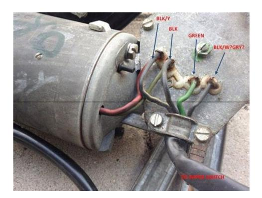
**4 wire wiper motor wiring diagram** is a crucial aspect for those who work on automotive systems, especially when it comes to repairing or replacing windshield wiper motors. Understanding the wiring diagram can aid in troubleshooting issues, ensuring proper installation, and maintaining the functionality of the wiper system. This article delves into the intricacies of 4 wire wiper motors, their wiring diagrams, and essential considerations for effective installation and troubleshooting.
