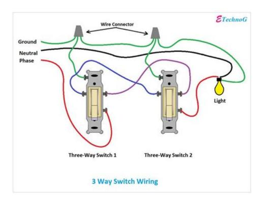
3 way switch wiring schematic diagram is an essential concept for anyone looking to understand residential electrical systems. A 3-way switch setup allows you to control a single light fixture from two different locations, providing convenience and flexibility in spaces like staircases, hallways, and large rooms. This article will delve into the intricacies of wiring a 3-way switch, including detailed explanations of the components, the wiring process, and safety considerations.
