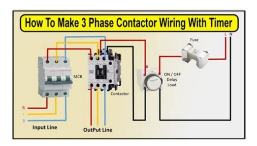
3 phase contactor wiring diagram with timer is an essential aspect of electrical control systems used in industrial and commercial applications. Understanding how to wire a three-phase contactor with a timer can enhance operational efficiency, automate processes, and ensure safety in electrical systems. This article provides a comprehensive guide to wiring a three-phase contactor with a timer, including its components, working principles, wiring diagrams, and practical applications.
