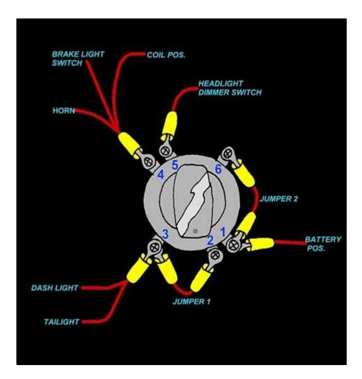
**6 pole ignition switch wiring diagram** is an essential component for anyone working on or understanding the electrical systems of vehicles, machinery, or other equipment that utilizes a multipole ignition switch. This article will delve into the significance of a 6 pole ignition switch, provide a detailed wiring diagram, and explain the various components involved in the setup.
