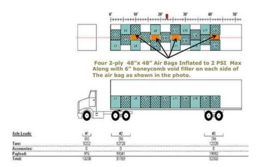
**53 ft trailer pallet loading diagram** is an essential tool for logistics and transportation professionals. Understanding how to effectively load a 53 ft trailer can significantly enhance efficiency, reduce damage during transport, and ensure compliance with weight regulations. This article delves into the various aspects of loading a 53 ft trailer, including optimal loading techniques, common pallet configurations, and tips for maximizing space.
