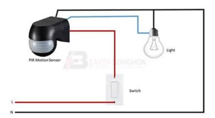
**4 wire motion sensor light wiring diagram** is essential for anyone looking to install a motion sensor light fixture effectively and safely. Understanding how to wire these devices correctly can save you time and prevent potential electrical hazards. This comprehensive guide will cover the necessary components, wiring process, and tips for troubleshooting common issues, ensuring your motion sensor light operates seamlessly.
